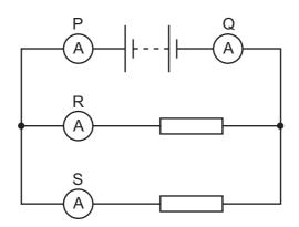
Which two ammeters read the largest current?
